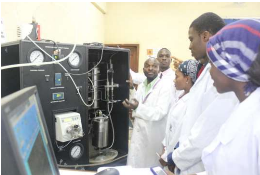
Figure 4.3: Demonstration of core flooding under reservoir and ambient conditions and determination of permeability with either liquid of gas.
